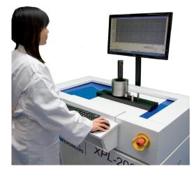
The MasterScanner is the only measuring machine in the world capable of a fully automated calibration, including all thread parameters of a part or a gauge in just a few minutes, and even compares the results with the dimensional tolerances of most popular standards. The MasterScanner is in many ISO 17025 accredited labs all around the world.
