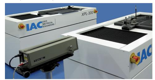
All MasterScanners are calibrated by laser interferometer for **highest accuracy and optimal traceability**
