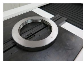
The MasterScanner is the only measuring machine in the world capable of a fully automated calibration, including all thread parameters of a part or a gauge in just a few minutes, and even compares the results with the dimensional tolerances of most popular standards. The MasterScanner is in many ISO 17025 accredited labs all around the world.
